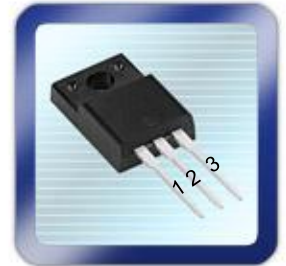
T0220 Full-PAK Isolated (T0-220) 1=Gate, 2=Drain, 3=Source
