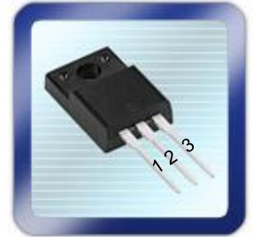
T0220 Full-PAK Isolated (T0-220) 1=Gate, 2=Drain, 3=Source
