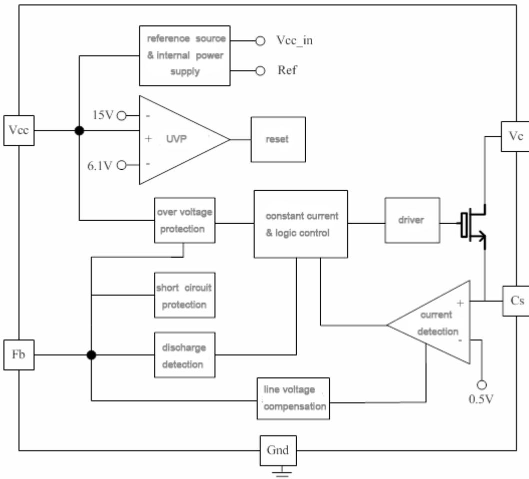
Picture 2 Internal Structure Diagram
