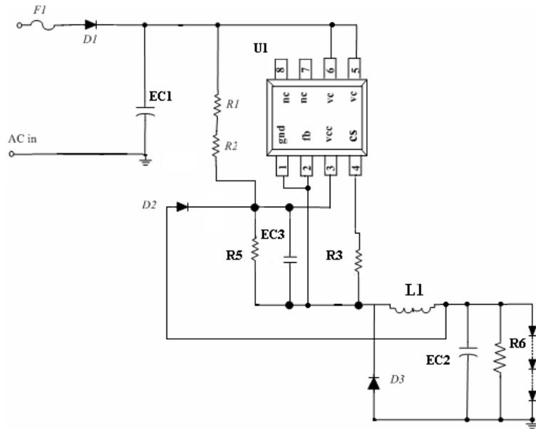
Picture 1 D80214 typical application schematic
