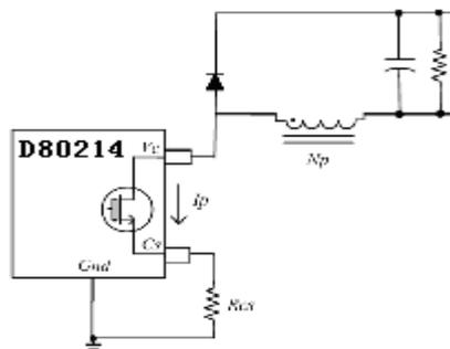
Picture 4 set constant current schematic
