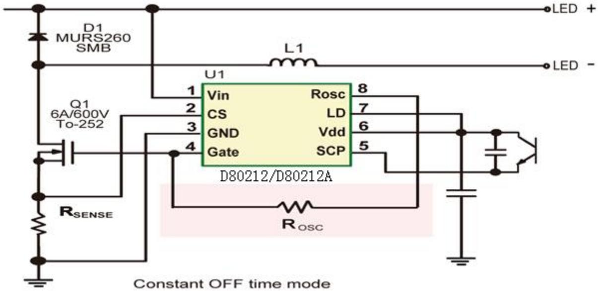
Figure 3: Typical Application Circuit (without PFC)
