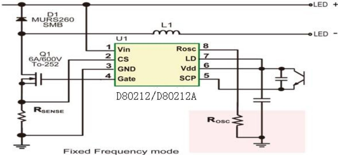
Benefiting from D80212 inherited high voltage feature, rectified DC high voltage ( $V_{DC} = V_{AC} \times 1.414$ ) can be directly fed into power pin of it to achieve high duty cycle, which is only limited by  $V_{OUT} / V_{IN}$ , to optimize design efficiency. This solution can easily achieve above 90% efficiency. However, if the duty cycle is configured to reach above more than 50%, some instability called sub-harmonics oscillation (SBO) will occur.
