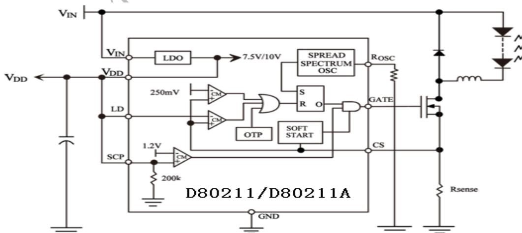
OTP: Over temperature protection at 125 $^{\circ}C$
