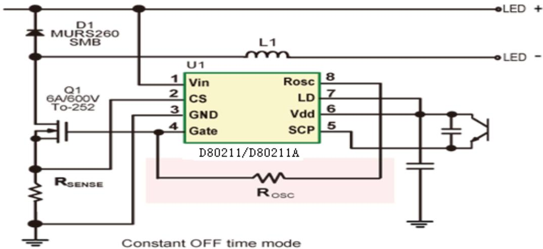
**Fig. 3: Typical Application Circuit (without PFC)**
